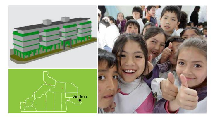
The project will be built on a piece of land with access to Belgrano street, as block modules or interconnected towers, both horizontally and vertically. The decision of projecting block or tower modules has to do with the potential for splitting construction and enlarging the building in several stages, while allowing for the independent operation of each of these modules.
